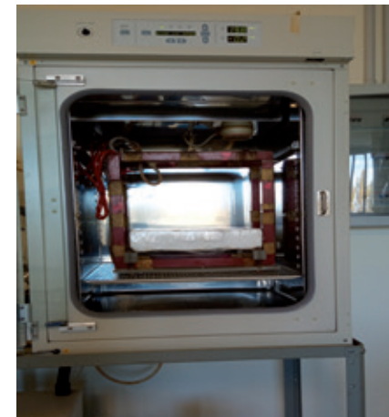
Extremely low frequency (50 Hz) magnetic field exposure system
